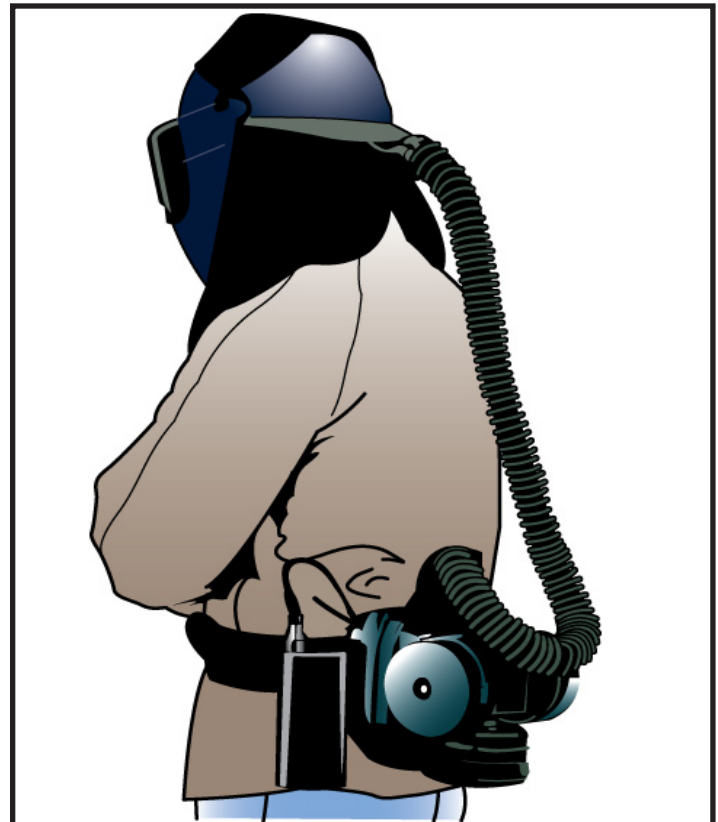
Figure 1.5 - Respirator with a Powered Air Purifier
