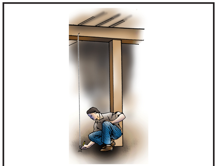
Figure I.15 - Using a Plumb Bob to Locate a Point
