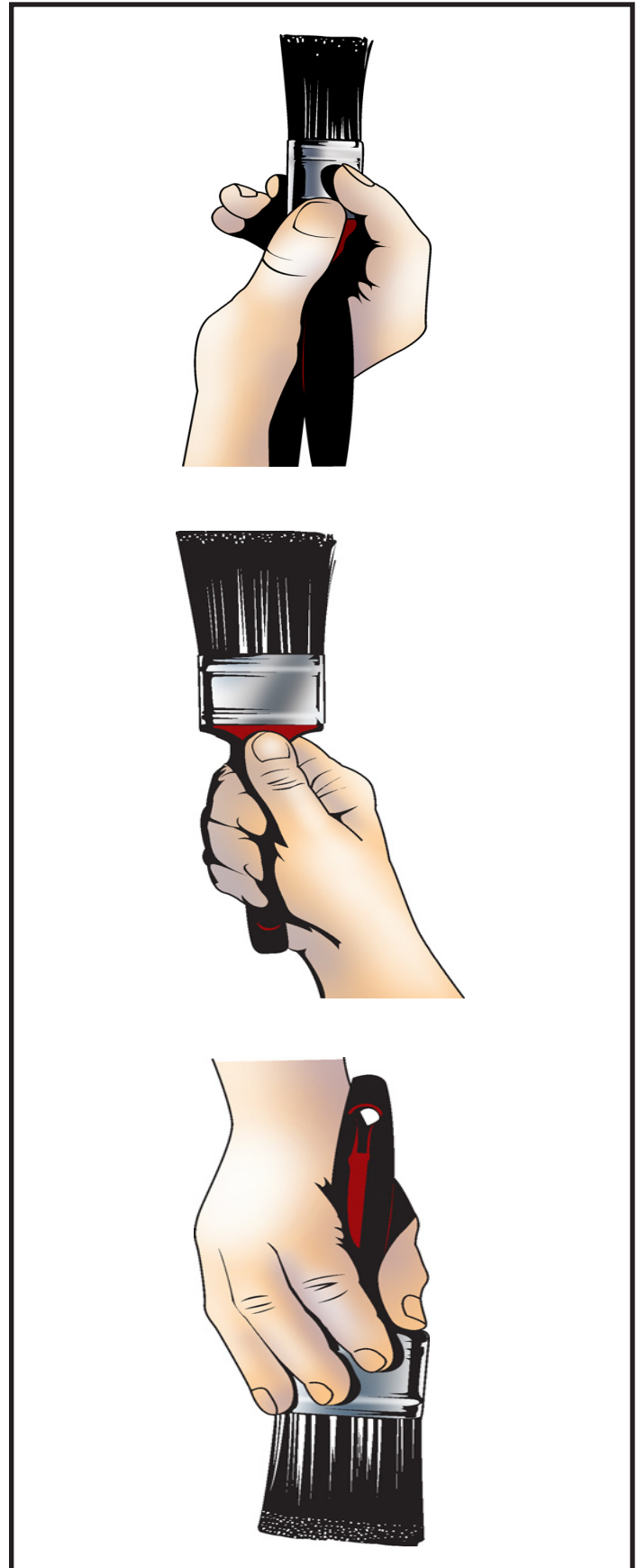
Figure 1.7 - Methods of Holding a Paintbrush
