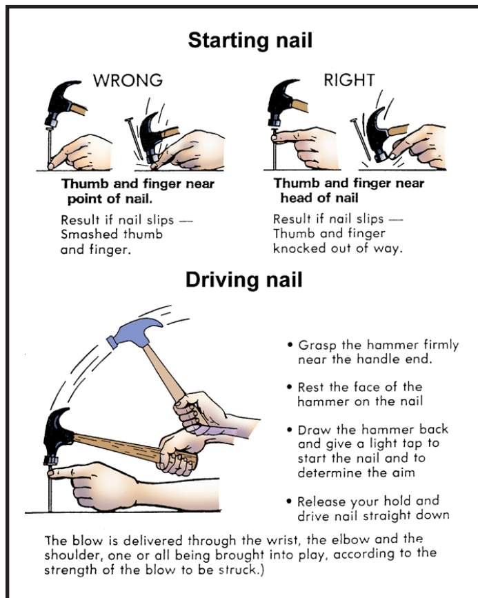
Figure 4.4 - Starting and Driving a Nail
