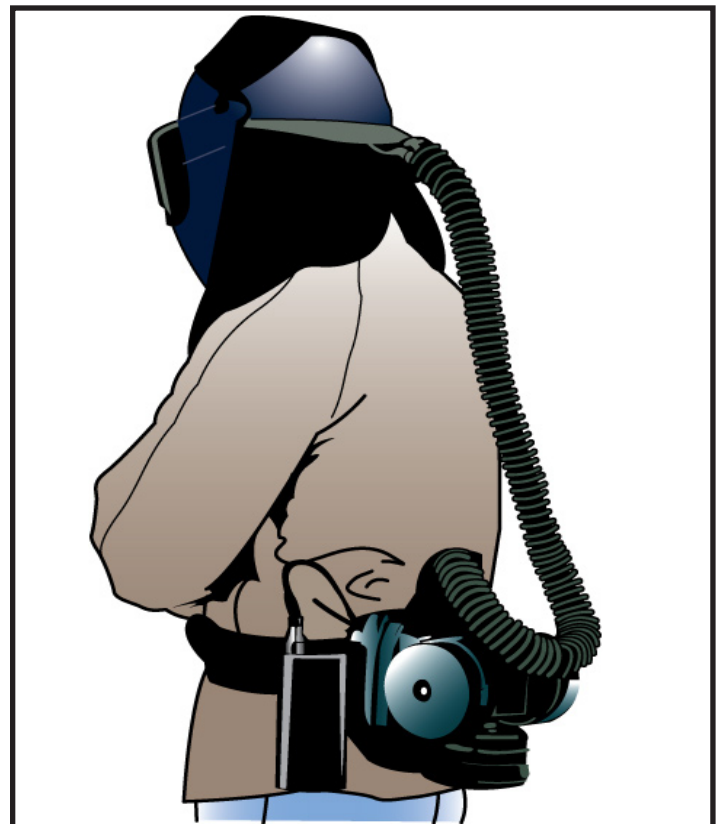
Figure 1.5 - Respirator with a Powered Air Purifier
