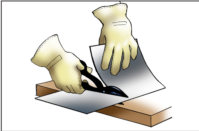
Figure I.4 – Lifting Metal Out of the Way When Using Snips to Cut Metal
