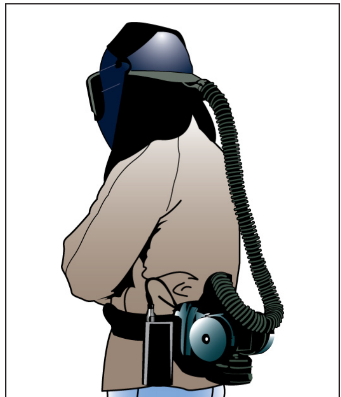
Figure I.5 – Respirator With a Powered Air Purifier
