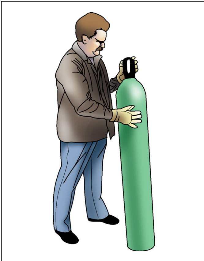
Figure 1.3 – Method of Moving a Cylinder
